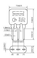
(1) : Input (2) : Ground (3) : Output (in mm)
