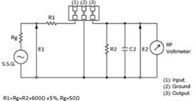
22=10pf (including stray capacitance and input capacitance of RF Voltmeter) E1: S.S.G. Output voltage
