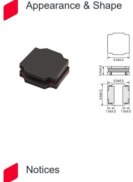
When rated current is applied to the products, inductance will be within ±30% of nominal inductance value. When rated current is applied to the products, temperature rise caused by selfgenerated heat shall be limited to 40°C max. Keep the temperature (ambient temperature plus selfgeneration of heat) under 125°C.
