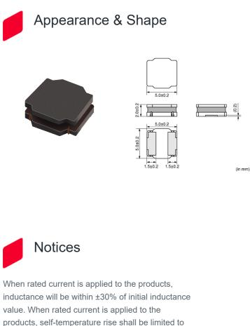
products, self-temperature rise shall be limited to 40°C max. Keep the temperature (ambient temperature plus self-generation of heat) under 125°C.
