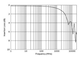
Common Mode Insertion Loss Characteristic (Typical Value)
