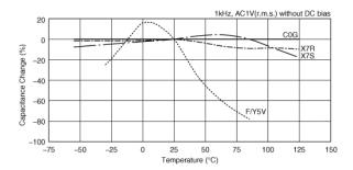
Capacitance - temperature characteristics
