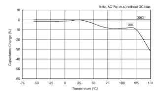
Capacitance - temperature characteristics
