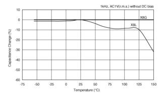
Capacitance - temperature characteristics
