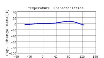
Temperature[degC] GRM155R70J105MA12 C-Temp. capchange, DC0.0V,
