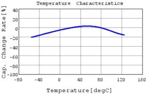
GRM21BC71C106KE11 C-Temp. capchange, DC0.0V,
