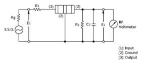
$Rg = 50\Omega$   $R_1 = 420\Omega \pm 5\%$   $R_2 = 470\Omega \pm 5\%$ C2 = 10 ± 2 pF (Including stray capacitance and Input capacitance of RF Voltmeter) E1: S.S.G. Output Voltage
