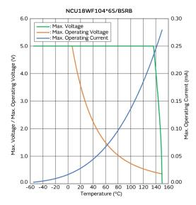
Max. Voltage, Max. Operating Voltage/Current **Reduction Curve**
