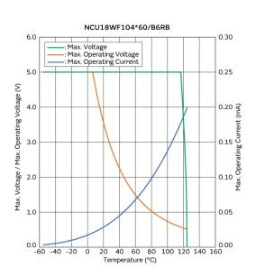
Max. Voltage, Max. Operating Voltage/Current Reduction Curve
