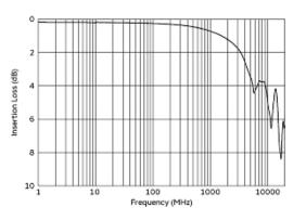
**Differential Mode Transmission Characteristics** (Typical Value)
