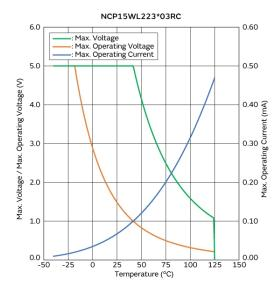
Max. Voltage, Max. Operating Voltage/Current **Reduction Curve**
