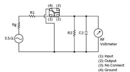
R1+Rg=R2=Input/Output Impedance, Rg=50Ω C2=10pF (Including stray capacitance and Input capacitance of RF Voltmeter) E1: S.S.G. Output Voltage Spurious Response
