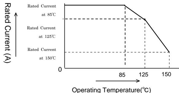
Keep the temperature (ambient temperature plus self-generation of heat) under 155°C.
