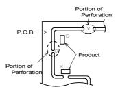
Products shall not be arranged on the line of a series of holes when there are big holes in P.C.B.
