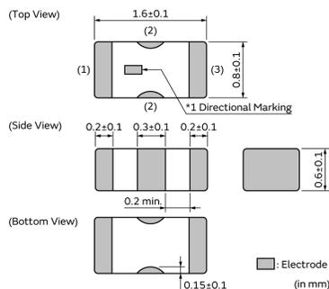
\*1 There is no electrical polarity, but there is a directional marking on the top of the product to identify inner physical direction.
