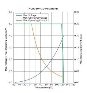
Max. Voltage, Max. Operating Voltage/Current Reduction Curve
