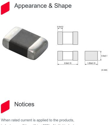
inductance will be within ±30% of initial inductance value range. When rated current is applied to the products, the temperature rise caused by self-generated heat shall be limited to 40°C max. Keep the temperature (ambient temperature plus self-generation of heat) under 125°C.
