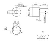
unit : mm Tolerance : ±0.3 Note: This datasheet may be out of date. Please download the latest datasheet of PV12P202A01B00 from the official website of Murata Manufacturing Co., Ltd.
