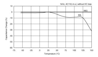
Capacitance - temperature characteristics
