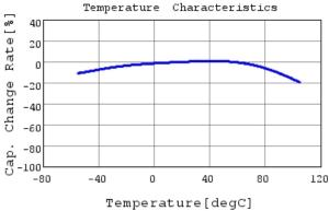
GRM21BC81C106KE15 C-Temp. capchange, DC0.0V,
