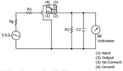
R1-Rg=R2=Input/Output Impedance, Rg= $50\Omega$ C2=10pF (Including stray capacitance and Input capacitance of RF Voltmeter) E1: S.S.G. Output Voltage
