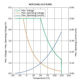
Max. Voltage, Max. Operating Voltage/Current **Reduction Curve**
