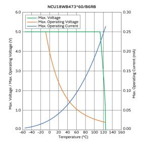
Max. Voltage, Max. Operating Voltage/Current **Reduction Curve**
