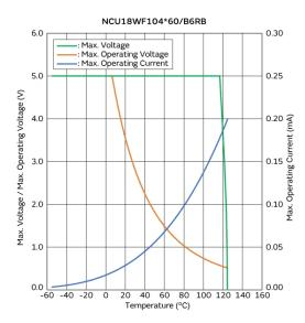
Max. Voltage, Max. Operating Voltage/Current **Reduction Curve**
