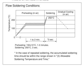
(5) There may be a risk of unexpected failures (tombstone, insufficient solder-wetting, etc.) in the mounting process caused by mounting conditions. Please make sure that this product is correctly mounted under the specified mounting conditions.
