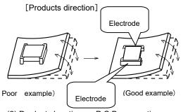
(2) Products location on P.C.B. separation Products (A,B,C,D) shall be located carefully so that products are not subject to the mechanical stress due to warping the board. Because they may be subjected the mechanical stress in order of A>C>B ≅ D. Products shall be located in the sideways direction (Length:a<b) to the mechanical stress.
