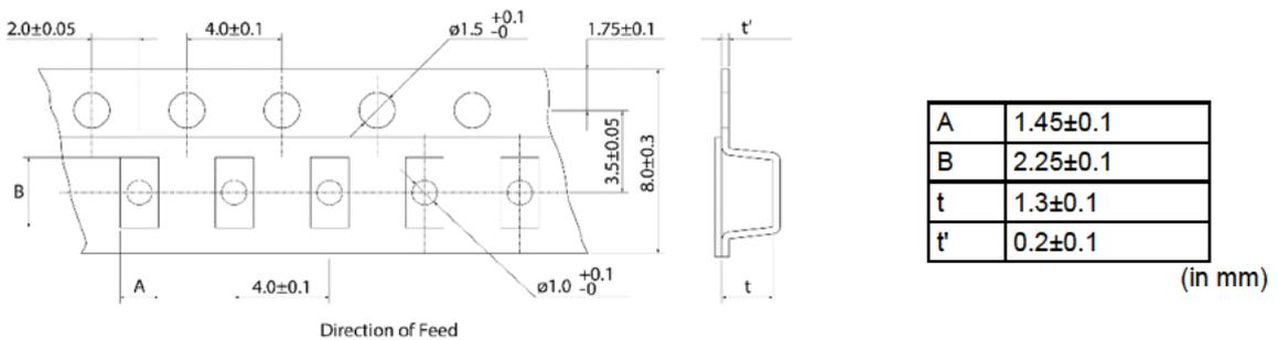
\* The dimensions of the cavity are measured at its bottom.
