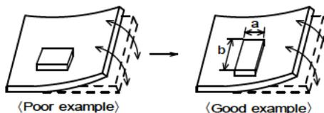
(2) Components location on PCB separation
