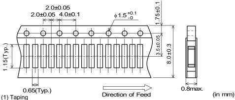
Products shall be packaged in the cavity of the base tape of 8mm-wide, 2mm-pitch continuously and sealed by top tape and bottom tape.
