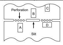
\*1 A > D is valid when stress is added vertically to the perforation as with Hand Separation.
