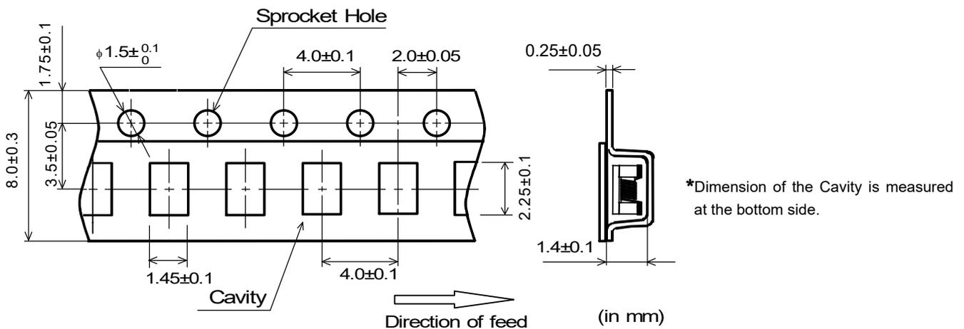
\*Dimension of the Cavity is measured at the bottom side.
