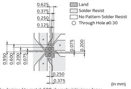
\* Line width to be designed to match 50Ω characteristic impedance, depending on PCB material and thickness.
