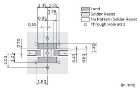
$<sup>^{\</sup>star}$  Line width to be designed to match  $50\Omega$  characteristic impedance, depending on PCB material and thickness.
