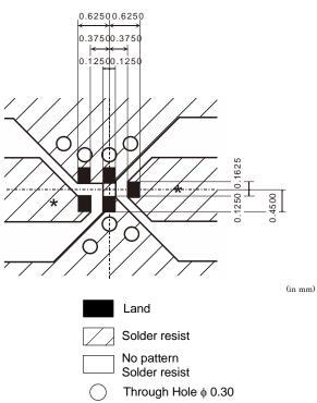
% Line width to be designed to match 50  $\Omega$  characteristic impedance, depending on PCB material and thickness.
