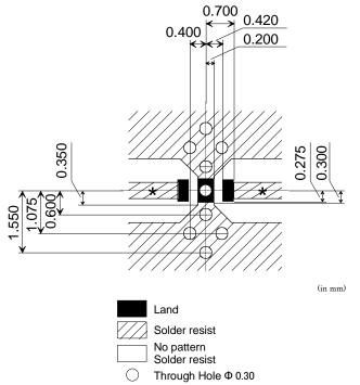
$<sup>^{\</sup>star}$  Line width to be designed to match 50 ohm characteristic impedance, Depending on PCB material and thickness
