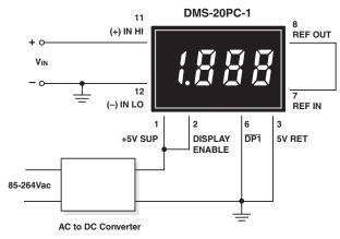
Figure 2. Single-Ended Input Configuration
