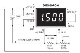
Figure 9. Basic DC Ammeter Circuit
