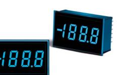
DMS-20PC Series, 3½ Digit, LED Display, Digital Panel Voltmeters combine a precision A/D converter; a factory-trimmed, highly stable, voltage reference; and a large (0.37"/9.4mm), easy-to-read LED display in a single package that is only slightly larger than the display itself. Displays are offered in either red, orange, amber, yellow, green or blue colors. High-intensity and low-power (35mW total) red LEDs are also optional.
