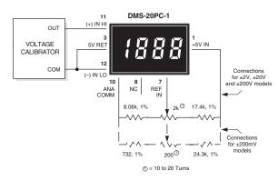
Figure 10. External Gain Adjustment
