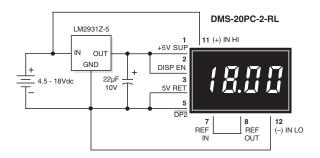
Figure 8. 4.5-18V Power Supply Monitor
