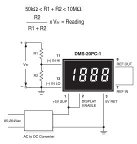
Figure 4. Input Attenuation Circuit
