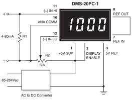
Figure 7. 4-to-20mA Current Loop Operation
