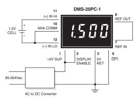
Figure 6. Floating Input Measurements (Alternate Configuration)
