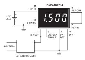
Figure 5. Floating Input Measurements
