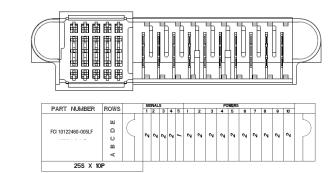
Note: "2" refers to the longest signal pin/power blade & "1" is the "shortest" signal pin such that the "shortest" is the "last to make, first to break" in the mating sequence.
