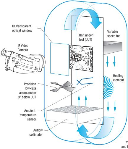
**Figure 8. Vertical Wind Tunnel**
