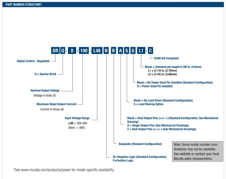
Regulated Quarter-Brick 800-Watt Isolated DC-DC Converter
