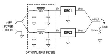
Figure 2. Load Sharing Block Diagram
