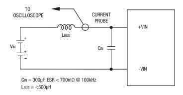
Figure 5. Measuring Input Ripple Current
