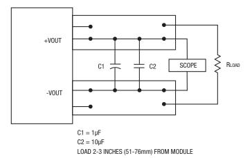
Figure 6. Measuring Output Ripple and Noise (PARD)
