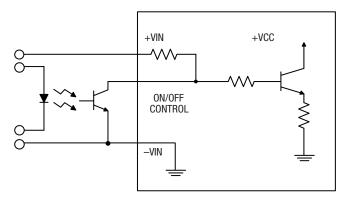
Figure 3. Driving the Negative Logic On/Off Control Pin
