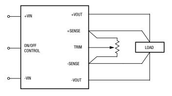
**Figure 6 Trim Connections Using A Trimpot**
