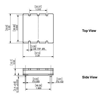
"V" Options Pins (Pin Option #1) with Slotted/Flanged Baseplate
