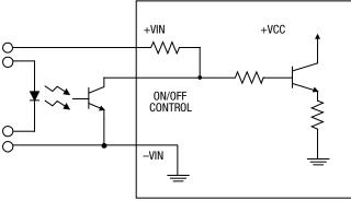
Figure 1. Driving the Negative Logic On/Off Control Pin
