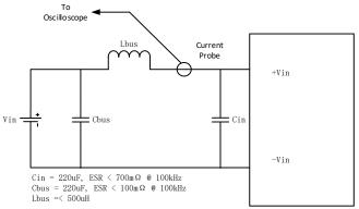
Figure 3. Measuring Input Ripple Current
