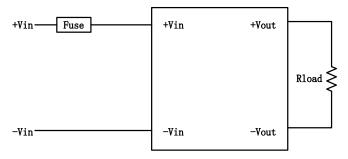
Figure 2. Input Fusing
