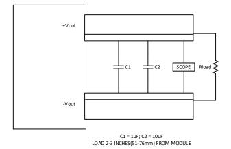
Figure 4 Measuring Output Ripple and Noise (PARD)
