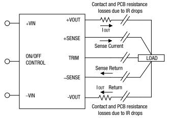
**Figure 5 Remote Sense Circuit Configuration**
