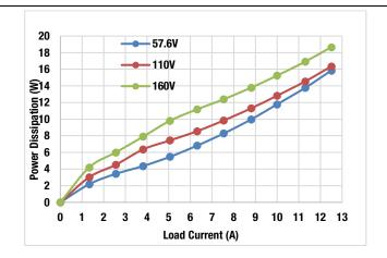
Power Dissipation vs. Load Current @25°C
