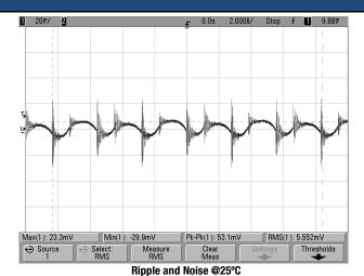
(Vin = 110V, Vout = nom., lout= 12.5A, Cload = 0, ScopeBW = 20MHz,  $2\mu$ S/div )
