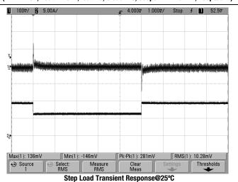
(Vin = 110V, Vout = nom., lout= 50-75-50% of full load, Cload = 0μF, ScopeBW =20MHz, 1mS/div)
