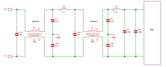
Figure 7. Conducted Emissions Test Circuit
