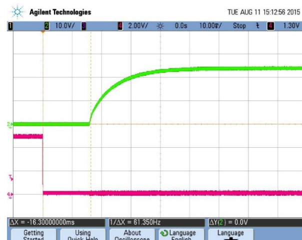
Turn-on transient at full load current (10 mS/div, Top Trace: Vout, 10V/div; Bottom Trace: ON/OFF, 2V/div)
