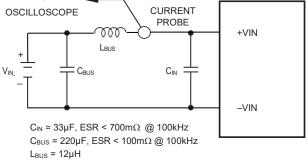
Figure 2. Measuring Input Ripple Current
