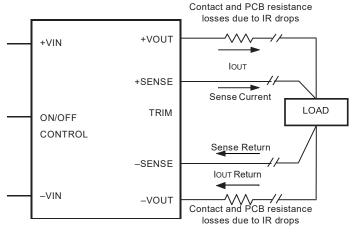
Figure 4. Remote Sense Circuit Configuration
