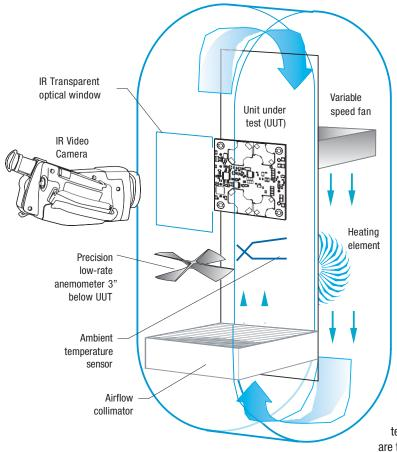
Figure 8. Vertical Wind Tunnel
