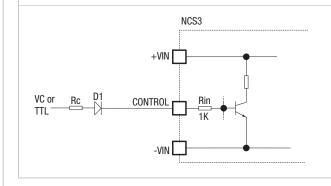
D1 (e.g. 1N4001) is necessary for correct operation of the NCS3 when the control signal is LOW. The recommended drive current Ig to shut down the NCS3 is 2 mA to 8 mA. The value of  $R_{\rm c}$  can be derived as follows:
