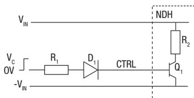
D<sub>1</sub> (eg 1N4001) is required to provide high impedance when the signal is low. From the NDH specification, the drive current to operate this function is recommended to be 6mA, and hence the value of R<sub>1</sub> can be derived as follows:
