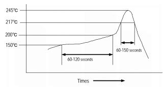
Do not vibrate for the products on reflow. Please need to take care temperature control because mounted parts may come off if the product is left under the high temperature. Do not mount on backside of the board.
