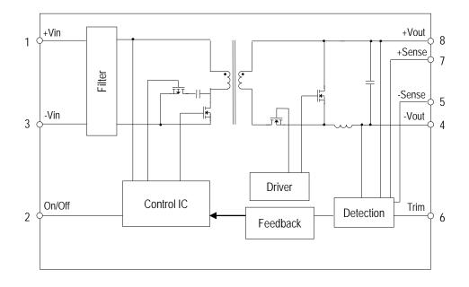
Figure 1. Simplified Block Diagram Typical topology is shown.
