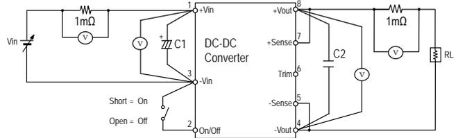
C1 : Low Impedance Electrolytic Capacitor 33μF
