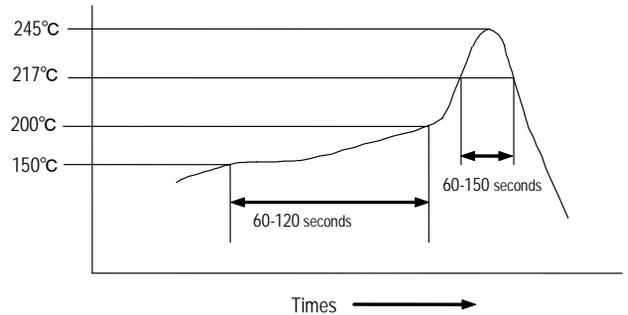
Do not vibrate for the products on reflow. Please need to take care temperature control because mounted parts may come off if the product is left under the high temperature. Do not mount on ackside of the board.
