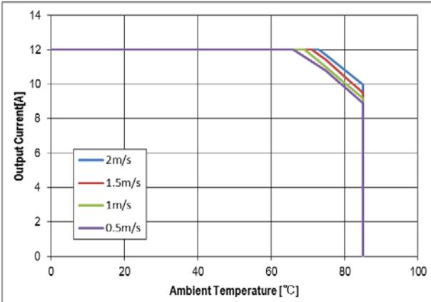
Thermal Derating (conduction cooling)
