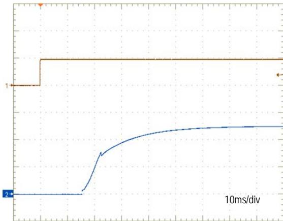
On/Off Enable Start-up ( $V_{in}=48V$ ,  $V_{out}=5V$ ,  $I_{out}=12A$ ,  $T_a=+25^{\circ}C$ )
