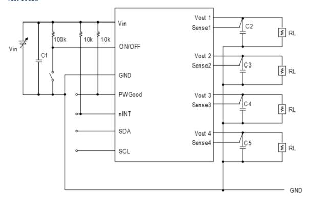
Vin: DC Power Supply RL: Electronic Load Device
