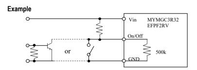
It is strongly recommended that on/off terminal should be used when you turn on/off this product. Characteristics may be affected by turning input voltage on/off.
